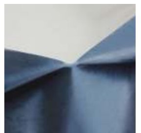
cross laminated film gap is hard to tear
