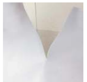
common HDPE film gap is easy to tear
